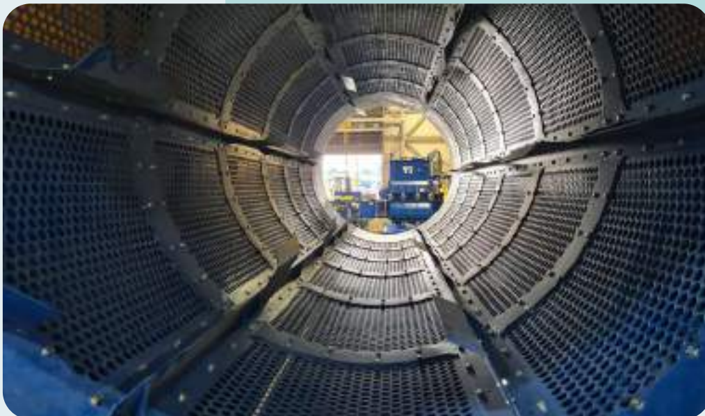
Image: Sherbourne Recycling's Trommel Screen for Size Sorting
